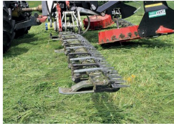
With the skids screwed at a height of 4-12 cm the cutting height can be varied
