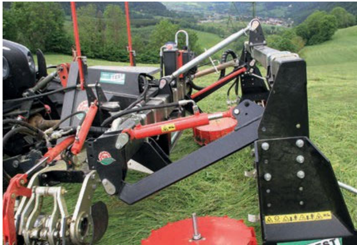
All mowing drives and hydraulic cylinders are supplied with on-board hydraulics with oil temperature monitoring and oil cooler.
