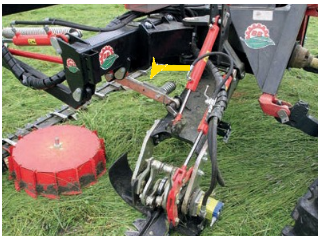
Collision protection for side outriggers (see arrow): In the event of overload, the rear mowers pivot 35° backwards.
