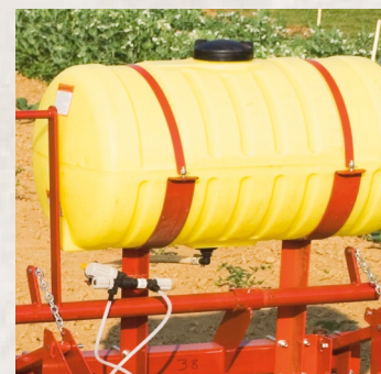
A gravity feed liquid side dresser option allows convenient application of fish emulsion or other liquid fertilizers. Poly tanks are available in #12-18 - One Row 25 Gal. #12-198 - Two Row 55 Gal.
